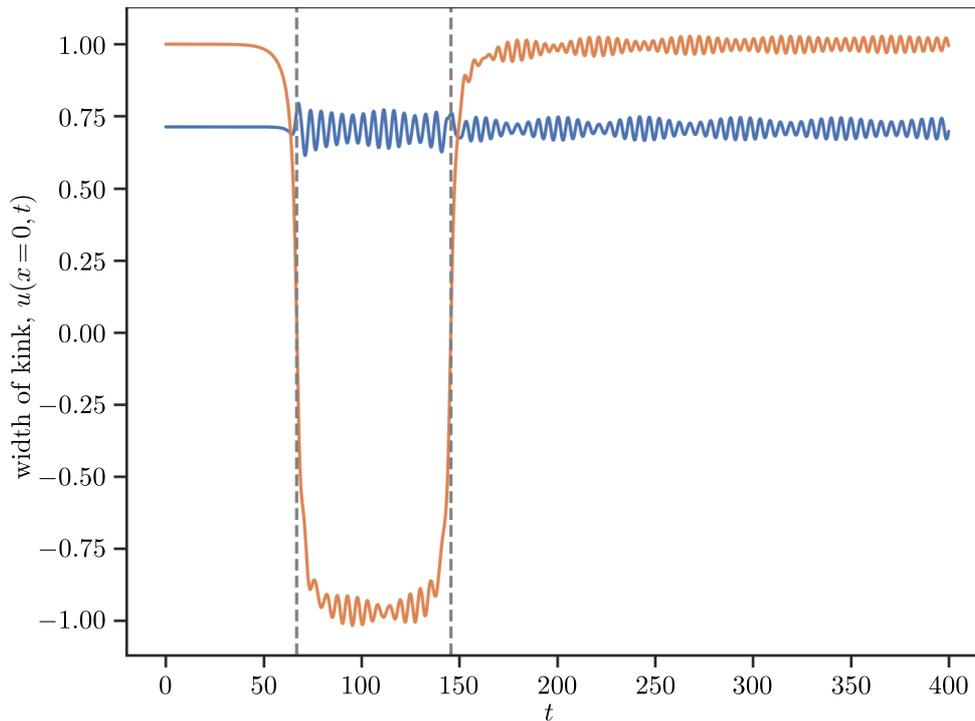
Fig. 15. Dependencies  $u(0, t)$  (red line) and  $u_x^{\max}(t)$  (blue line). Simulation parameters correspond to the resonant reflection of the kink by the potential well. Oscillations of  $u(0, t)$  reveal the excitation of the vibrational mode localized on the impurity, and oscillations of  $u_x^{\max}(t)$  reveal the excitation of the kink's internal mode. The moments of the first and second collisions of the kink with the potential well are shown by vertical dashed lines
