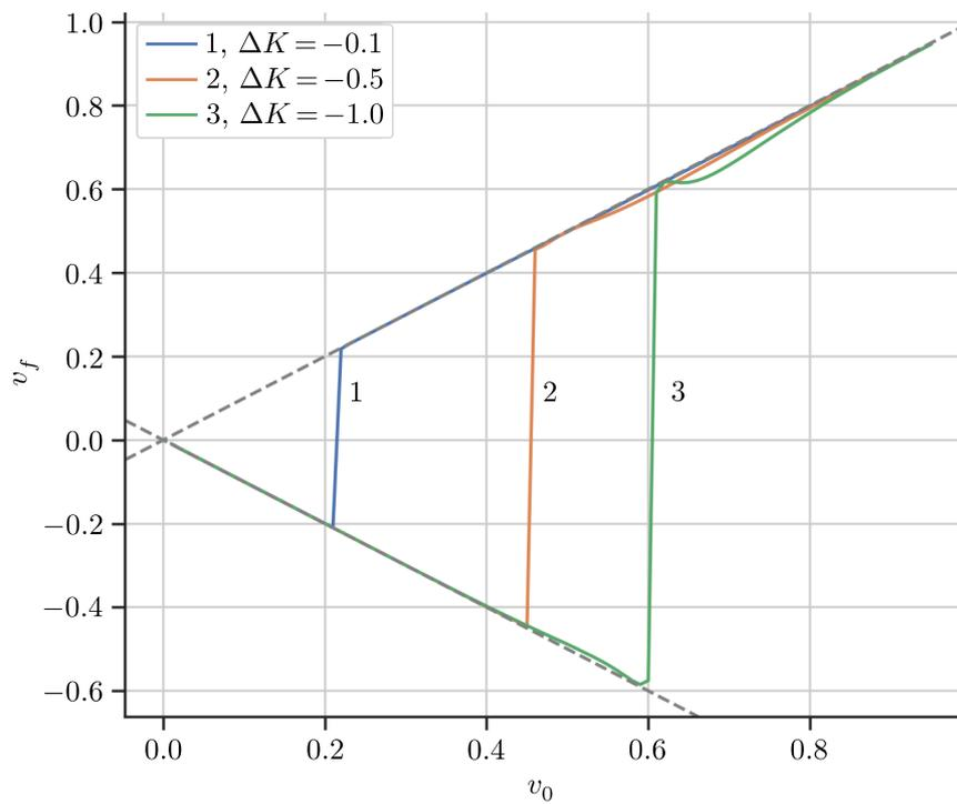
Fig. 4. Dependence of the final velocity of the kink after interaction with the barrier at different values of the parameter  $\Delta K$  for  $W = 1.0$
