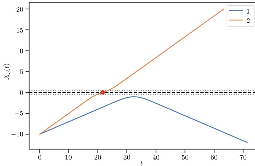
Fig. 1. Time dependence of the kink center coordinate,  $X_c(t)$ , at  $\Delta K = -0.5$  and  $W = 1.0$ . Curves 1 and 2 are for  $v_0 = 0.3$  and  $v_0 = 0.5$ , respectively. The dashed line shows the impurity center, the dotted lines show its boundaries
