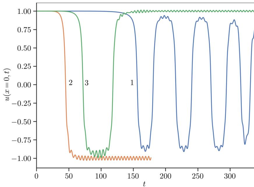
Fig. 8. Dependence  $u(0, t)$  for  $\Delta K = 0.5$ ,  $W = 1.0$  and initial kink velocities (a)  $v_0 = 0.05$ , kink pinning on the impurity, curve 1 (b)  $v_0 = 0.2$ , kink passage through the impurity, curve 2, and (c)  $v_0 = 0.11874$ , resonance reflection of the kink from the impurity, curve 3
