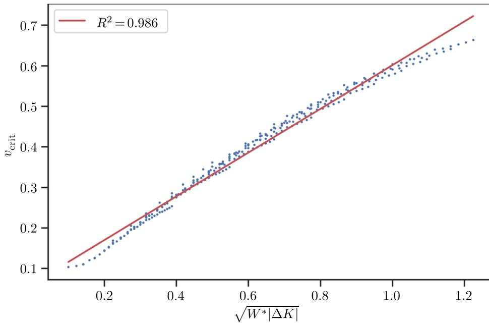
Fig. 3. Dependence of the critical velocity  $v_{\text{crit}}$  of impurity passage by a kink on  $\sqrt{W|\Delta K|}$  for  $\Delta K < 0$  (potential barrier). The critical velocity is nearly proportional to  $\sqrt{W|\Delta K|}$
