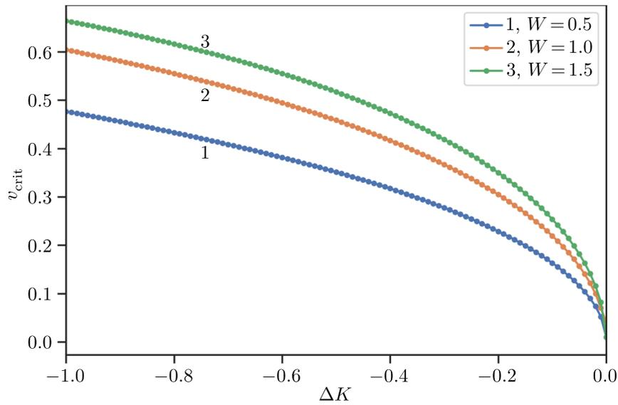
Fig. 2. Dependence of the critical velocity  $v_{\text{crit}}$  of impurity passage by a kink on the parameter  $\Delta K$
