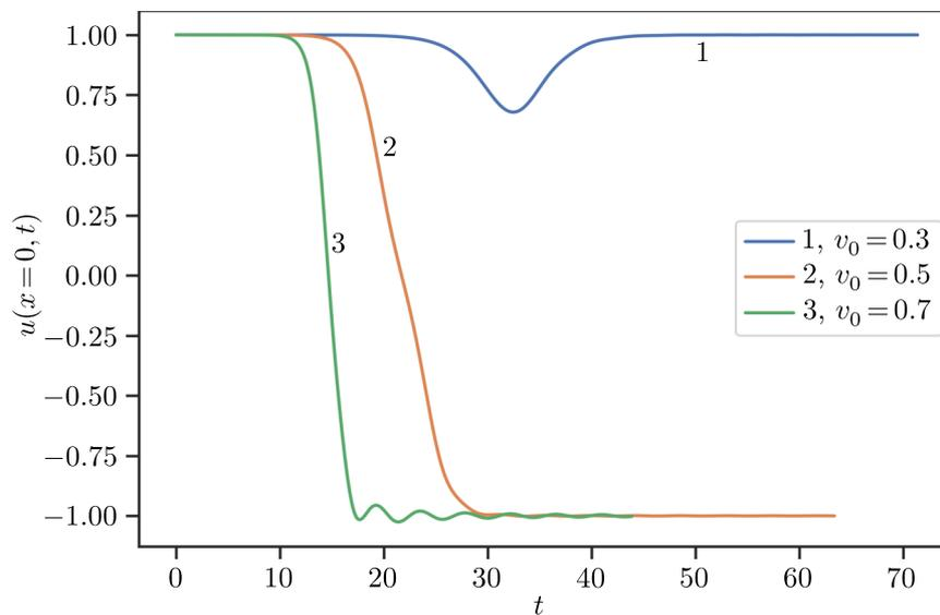
Fig. 5. Time evolution of  $u$  at the impurity center,  $x = 0$ , for different values of the initial kink velocity  $v_0$  for the parameters of the impurity  $\Delta K = -0.5$  and  $W = 1.0$
