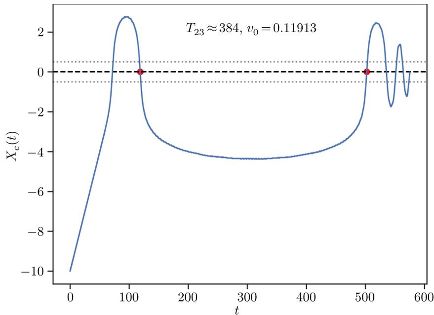
Fig. 14. Time dependence of the kink center coordinate at  $v_0 = 0.11913$ , which is close to the edge of the resonant reflection window
